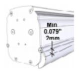
End stop is adjusted to allow the projection sheet to wind around the roller at least 1.5 times to avoid the sheet coming loose. Special attention must be paid when end stops are adjusted in such a way that projection sheet unwinds beyond the factory setting. Incorrect adjustment of end stops can cause:
