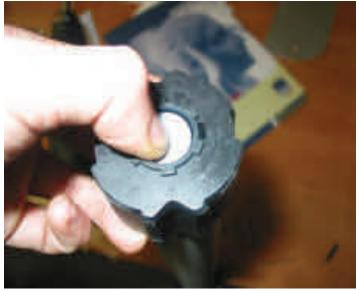
j) Please pull the cable back to it's position. Now it's possible to install the new motor inside the rolling tube like shown on the picture. It's very important to keep the right position of both rubber collars as shown on the picture below.
