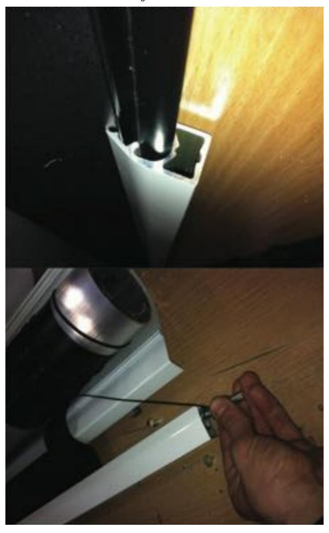
h) Remove the rubber collar from upper part of the motor. Push the plastic button in the front of the motor tube and pull it back as shown in the picture.
