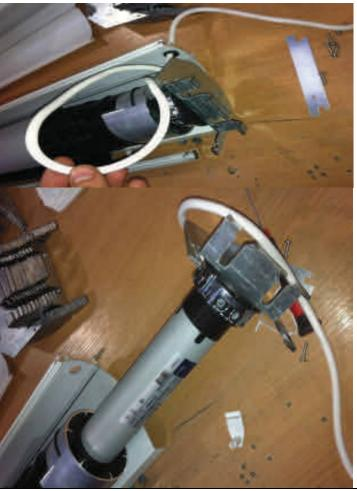
e) Now it's possible to remove both plastic end caps (left and right) from the batten and remove all batten from the fabric by sliding it on one side. Be sure that you have enough space to do this. Cut off nodes from the rubber strings on both sides and remove the metal pin. Remove metal clips from the iron bar and remove it from the fabric weld.
