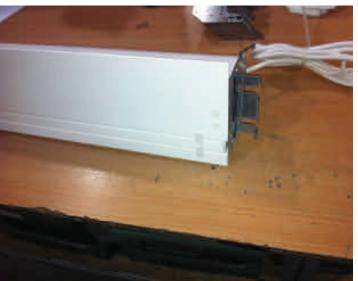
c) Depending on the type of the screen, unscrew screws on the both sides of the screen. The side parts of the screen and screws which have to be unscrewing are shown on the pictures below.
