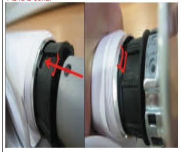
i) Install on the new motor all rubber collars (1 and 2). The correct position of rubber collar on the motor as shown below.
